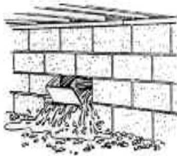
View From Inside Crawl Space - Door Pops Under Hydro-Static Pressures/Relieves Pressure On Foundation
